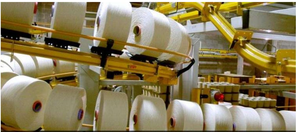
Installing Cone Collecting, Transport and Palletizing System means a considerable turning in Spinning Automation Process. The automation interfaces to productive line and involves Cone handling and packaging in a full autonomous way. In this phase of Industrial Automation, Trascar-
