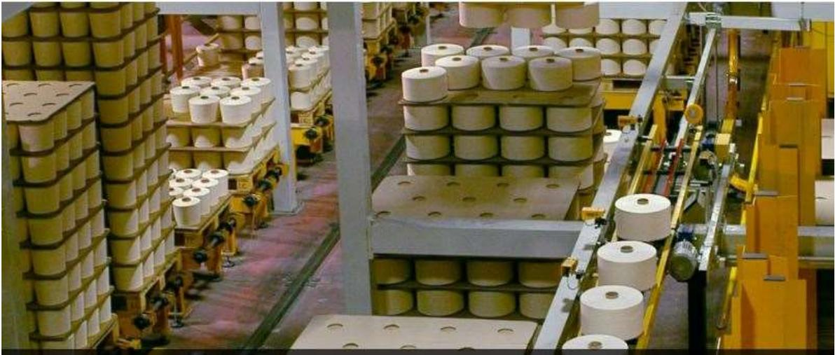
A Centralized Palletizer is equipped with several palletizing stations. The number of stations can be chosen according to the manufactured products varieties or the number of productive machinery.
