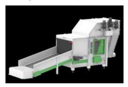
The Bale Opener ensures a gentle opening of strongly pressed fiber bales as well as a thorough mixing and equalization of the fibers. If required, the Bale Opener can be equipped with a weighing unit, mixing belt and Continuous Mixing Opener (CMO) for metering and mixing several fibre types.
